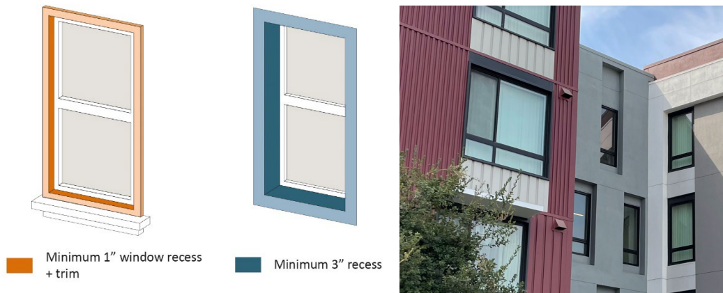
Figure 24.305.020.B-5. Window Trim or Recess
